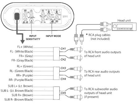
\* Using RCA plug cables (not included), connect RCA female connectors on the amplifier to the RCA audio outputs on your head unit. Make sure the left and right channels are correctly matched. To reduce the possibility of noise entering signal chain, use high-quality RCA cables for better insulation and run the RCA cables away from large wire loops, electric fan and power wires.
