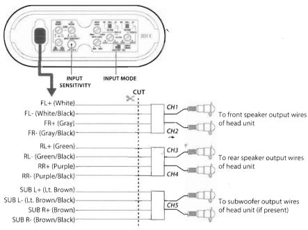
As illustrated above, cut off the RCA female connectors so that the supplied input harness can be used for high-level input. Then connect the colored wires to speaker output wires of your head unit. Observe speaker polarity. Make sure the speaker wires are securely connected and properly insulated.
